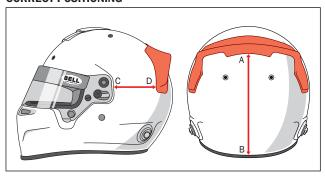
Take points of reference by measuring the position of the spoiler as shown on the diagrams and according to your helmet size. (See chart below)
