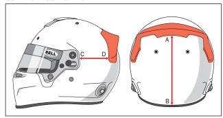
Take points of reference by measuring the position of the spoiler as shown on the diagrams and according to your helmet size. (See chart below)
